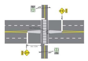
Guideline 24: At-grade mid-block multi-use pathways crossings collector and arterial roadways should be controlled by a pedestrian signal or pedestrian crossover where possible. The midblock pedestrian signal is a device to assist pedestrians crossing major streets and is a more positive and effective pedestrian crossing device than a pedestrian crossover (PXO).
