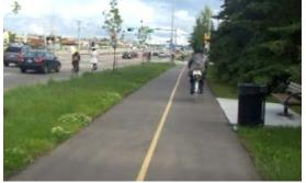
The Boulevard Multi-use Trail or "Active Transportation Pathway" is a facility that is **within the road right-of-way** but is physically separated from motor vehicle traffic by a landscape buffer or "verge".
