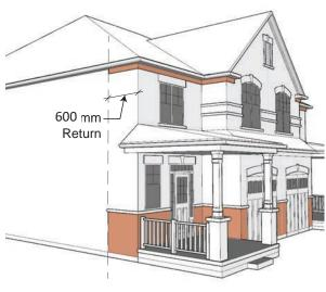
Front façade detailing (i.e. stone, stucco, frieze/cornice) shall return a minimum of 600mm along the side wall
